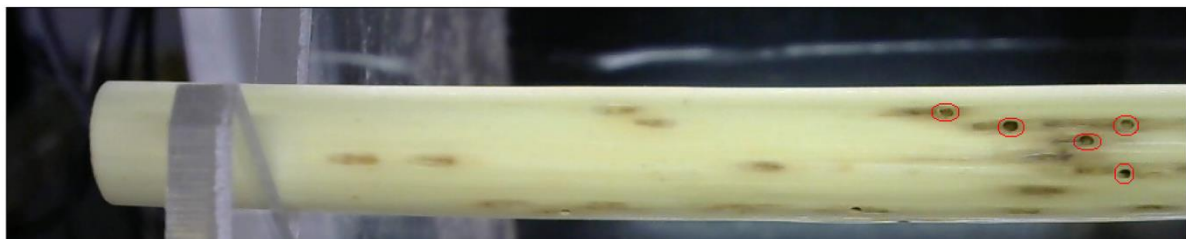
(b) Defect class: circle holes
