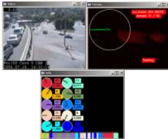
Fig. 5. Sample frame (top left); flow field and direction histogram (top right: red is the mean motion field, green is the directional histogram of the current sample); bottom: directional classes, with colored circles as the class mean.
