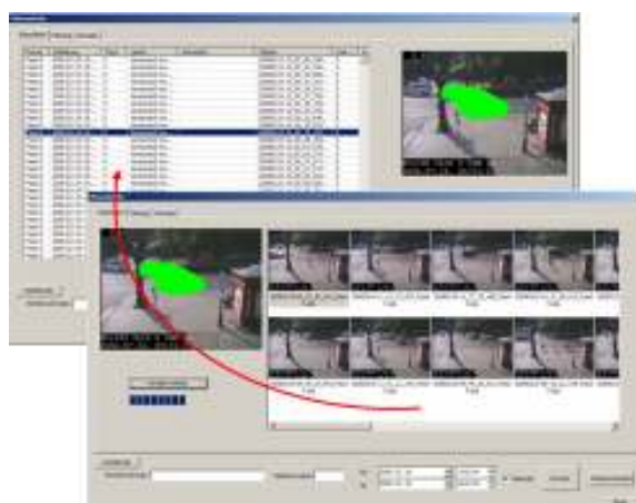
Fig. 17. Browsing by selecting region of interest: select a region, search, browse through results, then view associated alert details by double clicking.
