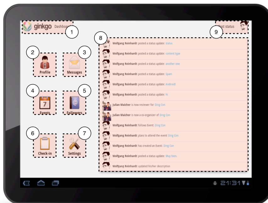
Figure 6 Main elements of the ginkgo mobile interface (on Android 3)
