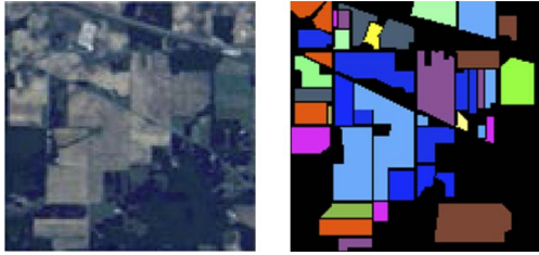
Fig. 7. Indian Pines data set. (Left) False color composite image (bands 28, 19, and 10) and (right) ground truth.
