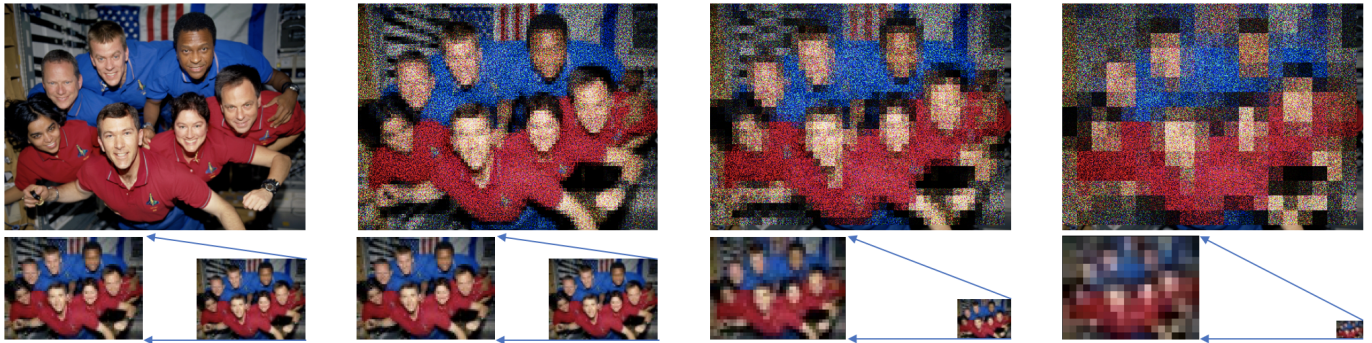
Fig. 2: TPE-encrypted images with different block sizes (original, 5 \times 5 , 10 \times 10 , 20 \times 20 ), and corresponding preserved thumbnails.
