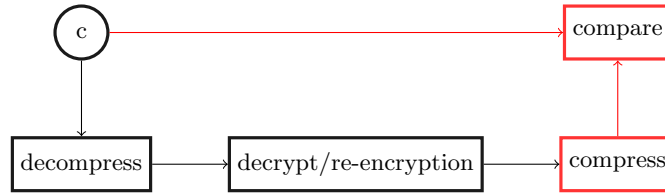
Fig. 1. Visualisation of the FO-transforms re-encryption check including decompression and compression. Being able to introduce one-bit faults anywhere in the red (light) phases enables our attack.
