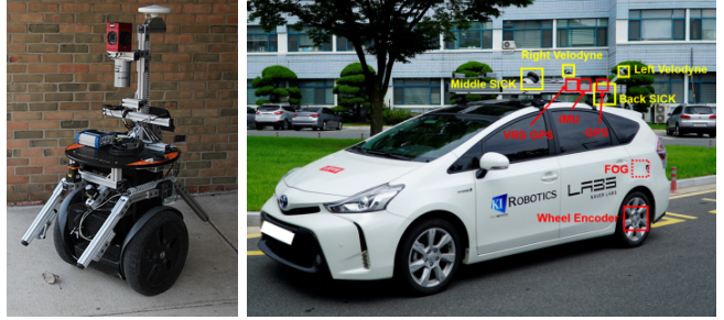
Fig. 1. The considered datasets [18] (left) and [19] (right) contain data logs of two wheel encoders, a fiber optic gyro and a consumer IMU, recorded, respectively on a Segway and a consumer car.
