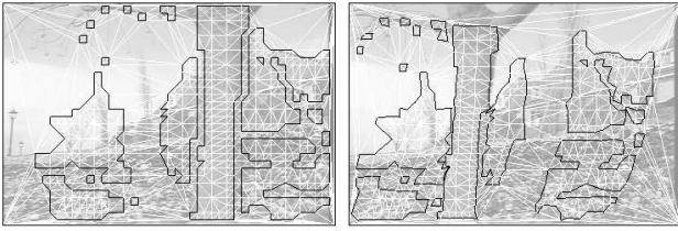
Figure 7. The result of the joint view triangulation: the black edges are the boundary edges of the matched regions and the white edges are Delaunay edges which are not matched.
