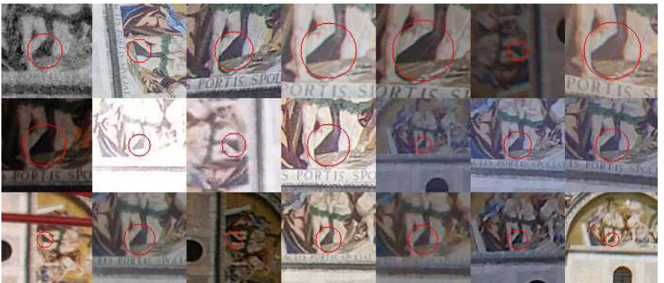
Fig. 2. Some of the keypoints from the same 3D point for the Venice data set in Fig. 16 are shown as an example. The red circle shows the keypoint (DoG) position and its scale. The track was extracted by consecutive SIFT L_2 matching, which makes it possible to include keypoint pairs (conjunctive closures) that are quite different into the training and evaluation set.
