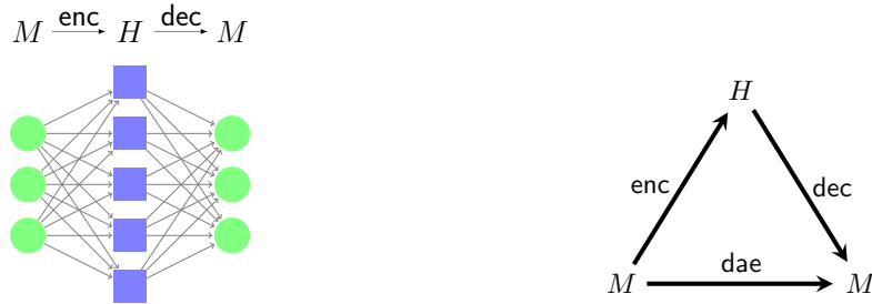
Figure 11: \text{enc} and \text{dec} correspond to the hidden layer and output layer, respectively.
