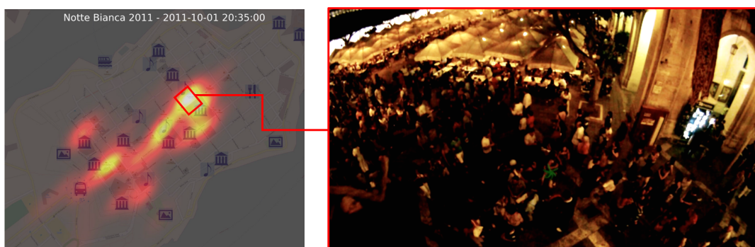
FIGURE 3.6: Crowd density estimation compared with ground truth video footage recorded during the 2011 Notte Bianca festival in Valletta, Malta
