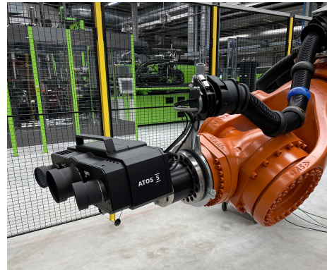
(b) Using the ATOS5 mounted on the robots.
