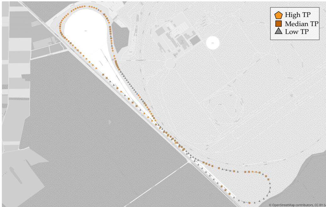
FIGURE 3.3: Throughputs (TPs) of a test round in Dudenhofen, separated into three classes with equal number of items and then drawn into the map. It can be seen that the Throughput (TP) has a correlation to the location as neighbouring measurement points tend to be in the same class. The map is based on Open Street Map (OSM) [162] data.
