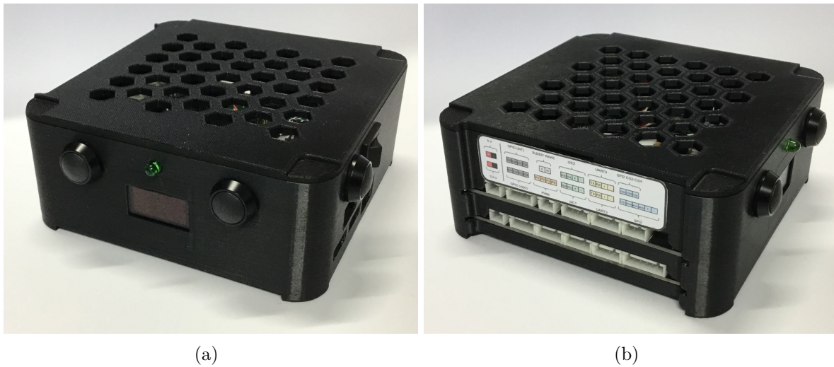
Figure 6.19: Images of the advanced Model-Testbed based on the STM32L476 showing the front (a) and side (b) of the 3D-printed enclosure.
