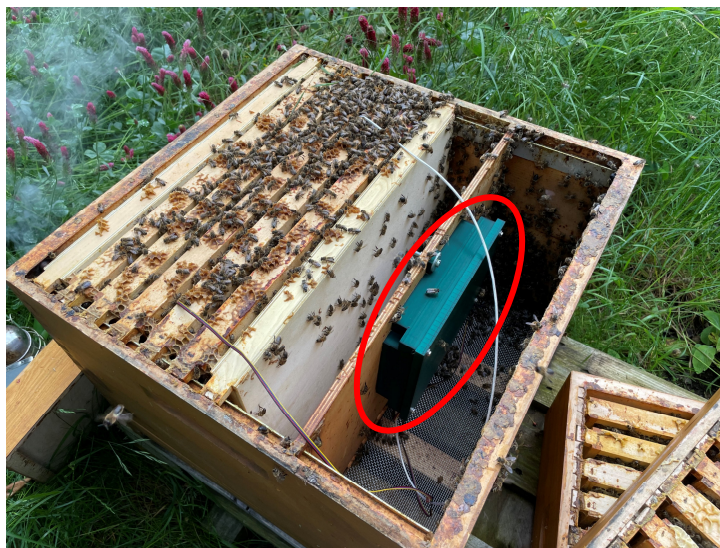
Figure 7.3: The prototype microclimate sensor node applied in a beehive (red circle).
