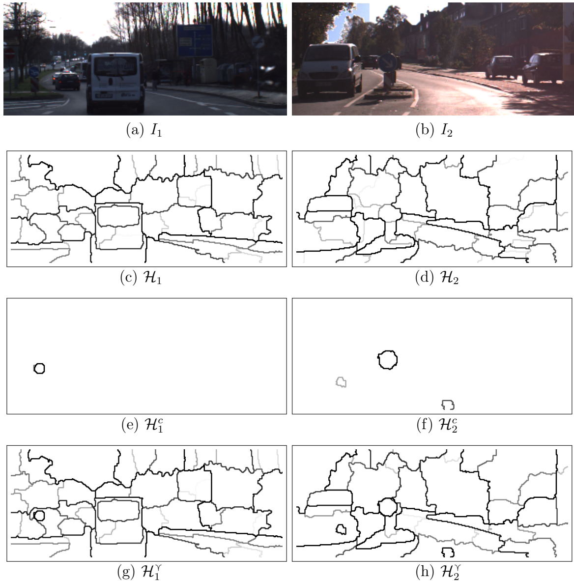
Figure 7.14: (a) and (b): original images from the German traffic sign dataset [49]. (c) \mathcal{H}_1 : area-based hierarchical watershed computed of the SED gradient of I_1 . (d) \mathcal{H}_2 : area-based hierarchical watershed computed of the SED gradient of I_2 . (e) \mathcal{H}_1^c : circularity based hierarchy computed from the regions of the dynamics-based hierarchical watershed of the SED gradient of I_1 . (f) \mathcal{H}_2^c : circularity based hierarchy computed from the regions of the dynamics-based hierarchical watershed of the SED gradient of I_2 . (g) \mathcal{H}_1^\gamma : combination of \mathcal{H}_1 and \mathcal{H}_1^c by supremum. (h) \mathcal{H}_2^\gamma : combination of \mathcal{H}_2 and \mathcal{H}_2^c by supremum.
