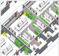
The mini-labs are designed to support the operations of up to three distinct entities or researchers with a common/shared area for equipment. Each of the approximately 1,000-square-foot labs is equipped with the following amenities:
