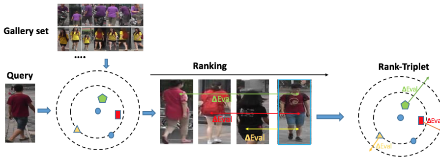
Fig. 1: Schematic illustration of Rank-Triplet. An image of a person of interest on the left (the query) is used to rank images from a gallery according to how closely they match that person. The correct match, highlighted in a blue box, can be difficult to find given the similar negative images, pose and viewpoint variations and occlusions. During training, we propose to estimate the importance of mis-ranked pairs by the gain of the evaluation measure incurred by swapping the rank positions and to weight the loss according to their importance. In this example, swapping the falsely ranked (positive) image on the right with the leftmost one would lead to the biggest improvement ( \Delta Eval ).
