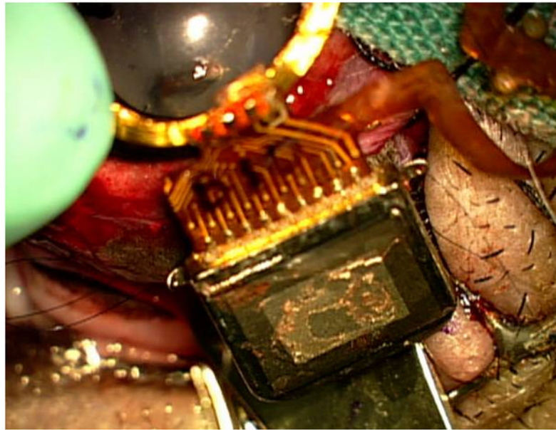
Fig. 9. Photo of the surgical implantation of a hermetic prosthesis onto the minipig eye. The molded gold telemetry coil surrounded the cornea, while the titanium hermetic case containing the custom stimulation electronics was attached to the sclera. The conjunctiva was later sutured over the implant to maintain sterility.
