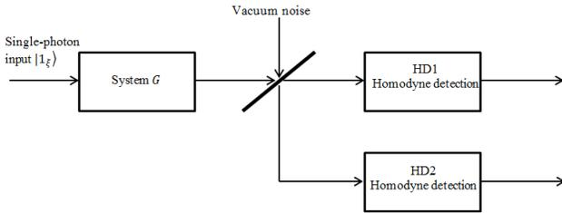
Fig. 3. Both homodyne detection measurements at the outputs of a beam splitter in quantum system.
