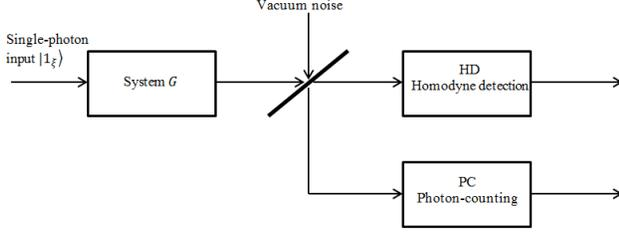
Fig. 1. Simultaneous homodyne detection and photon-counting at the outputs of a beam splitter in quantum system.
