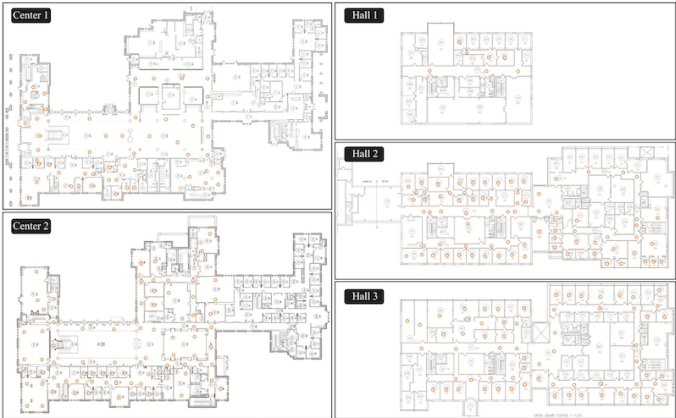
Figure 2: We have used a professional grade laser range finder to acquire building-scale panorama RGBD scans over five floors in two buildings. An orange circle indicates a rough scan location. Only one scan has been acquired in each room in most cases, making the intersection of adjacent scans minimal and the use of floorplan-image essential for our problem.
