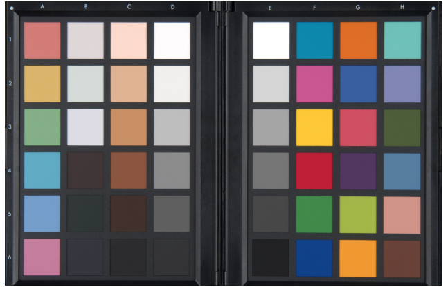
Figure 6. Test scene used for noise parameter calibration.
