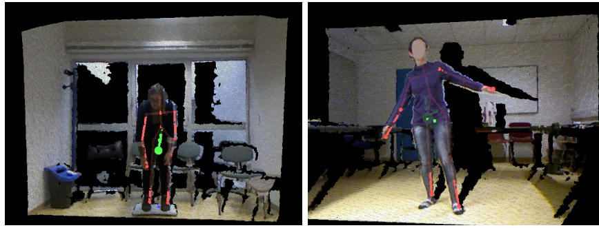
Fig. 3. 3D visualization of CoM based on SESC with Kinect user tracking.
