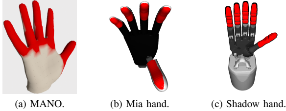
Fig. 9: Contact surfaces of the MANO model and the robotic hands are marked in red color.
