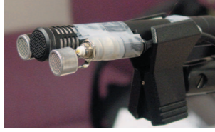
Fig. 1. The Doppler-augmented microphone used in our experiments. The two devices taped to the sides of the central audio microphone are a high-frequency emitter and a high-frequency sensor.
