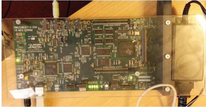
Fig. 1: Texas Instruments TMS320C6713 floating point digital signal processing platform.
