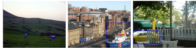
Figure 1: Left: detecting the sheep on this scene is very difficult without referring on the context, mountainish landscape. Center: In contrast, the context on the right image can only confuse the detection of the boat. The pure object characteristics is what a recognition model should focus on in this case. Right: This car instance is occluded on its right part and the recognition model should focus on the left part in order to confidently detect it.
