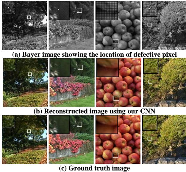
**Figure 5: Test results for defect pixel correction: (a) shows the location of the defective pixel with a white dot inside the white rectangle. A zoomed in view of the defect pixel region is shown in the top left hand corner in (a), (b) and (c).**
