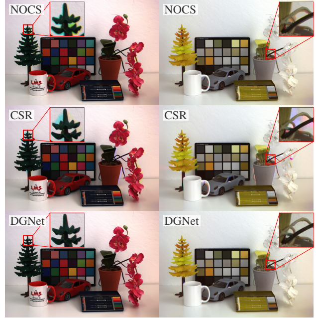
Fig. 4. Reconstruction results of spectrally guided methods as (false) color images combining three spectral bands. Left column: center row of camera array (red, green, blue). Right column: top row of camera array (infrared filters at 750 nm, 850 nm and 950 nm). Zoomed areas are depicted using red rectangles.
