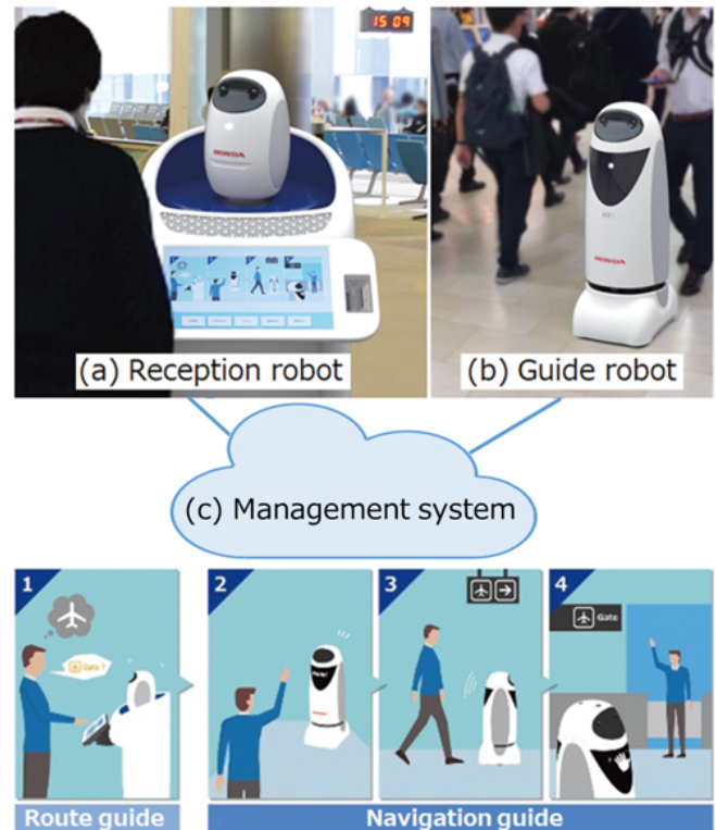
Fig. 1. Stationary reception robots in charge of the initial user interaction and mobile guide robots, executing the guiding task, efficiently collaborate under our newly designed management system.
