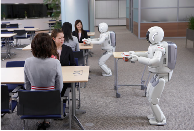
Fig. 2. Multiple ASIMO serves drinks to the guests. The cooperative work function enables tasks to be performed cooperatively. A server tracks task status of each ASIMO and distributes tasks to them optimally.
