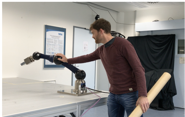
Fig. 9: The robot is pushed at joint 3 and 4 (collision 2).
