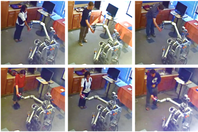
Fig. 8. Handing configurations chosen for comparative evaluation on the physical robot. (Top) Learned hand-over configuration for the bottle. (Bottom) Planned hand-over configuration for the mug.
