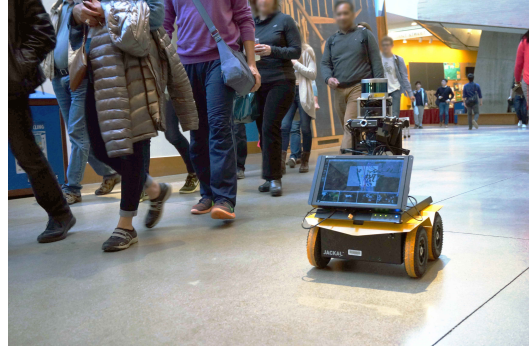
Fig. 1: A robotic vehicle navigating autonomously in a pedestrian-rich environment. Accounting for social interactions is important for operating such vehicles safely and smoothly.
