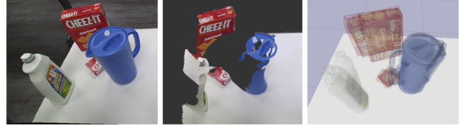
Fig. 1. Left: An RGB image for a scenario considered in this work. The target “Jell-o” object is located between and in close proximity to other objects. Center: Point cloud obtained from the RGB-D sensor highlighting the occlusions and partial object views. Right: Example output of pose estimation returning a discrete set of poses for objects in the scene.
