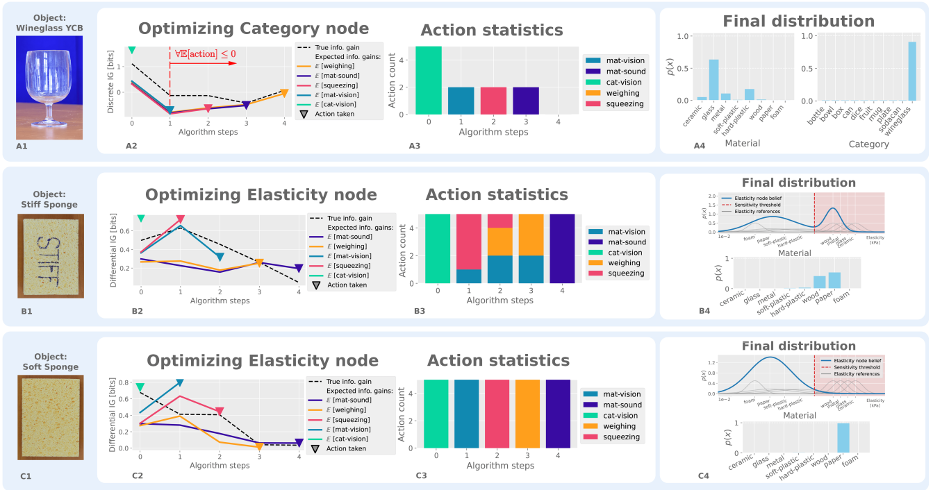
Fig. 5: System operation and performance – examples. (Left – A1/B1/C1) Object name and image. (A2/B2/C2) Single run of experiment with termination criterion off. Expected IG of the actions shown. Triangle markers show which action was chosen in a given step. The dashed black line shows the experimental true IG after the action was executed. This action is not shown anymore in subsequent algorithm steps. (A3/B3/C3) Count of actions chosen during the runs with the termination on (if all available actions at a given step had negative expected IG, execution stopped). (A4/B4/C4) Probability distributions of relevant variables of the single run shown in (A2/B2/C2).
