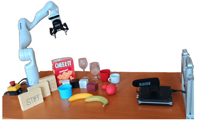
Fig. 4: All 17 objects used and experimental setup. Kinova Gen3 robot, Robotiq 2f-85 gripper, Rode VideoMic Pro microphone, and RealSense D435 camera (on the right; only the RGB from one camera was used).
