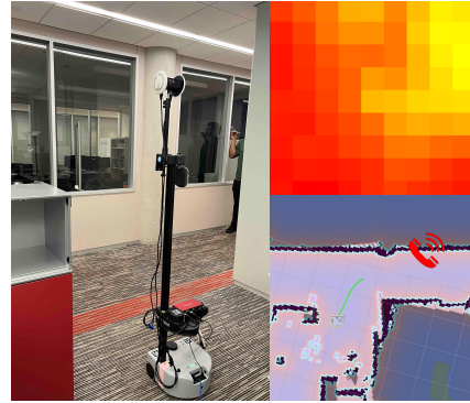
Fig. 1: Our robot predicts an acoustic field with a frequency-adaptive model and navigates to locate the sound source.
