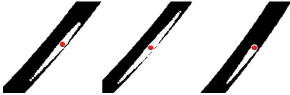
Figure 9: A view of the obstacle expansion in the grid with V_1 = 20m/s and V_2 = 5m/s in the left, V_2 = 10m/s in the middle and V_2 = 0m/s in the right
