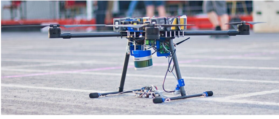
Fig. 11: A custom built quadcopter equipped with a Velodyne VLP-16 LiDAR sensor
