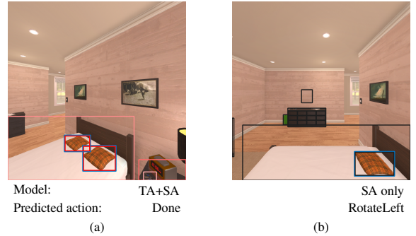
Fig. 5. The comparison of TDANet and the SA-only network for unseen object goal navigation. The target object Pillow is marked with the blue bounding box. (a) TDANet predicts the right action by focusing on objects related to the target. (b) Without the help of the TA module, the SA-only network is distracted by unrelated objects and predicts the wrong action.
