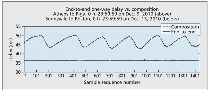
Figure 3. Comparison between the end-to-end delay measurement and composition.
