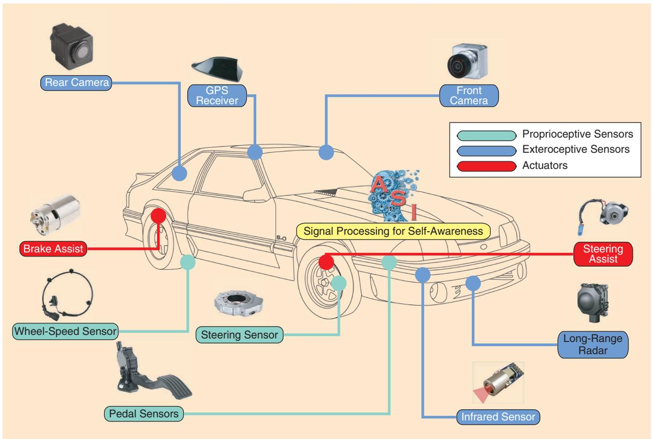
**FIGURE 1.** An architecture for a self-aware autonomous system. The autonomous vehicle observes the surrounding environment with exteroceptive sensors (blue) and its internal state with proprioceptive sensors (green). It translates its autonomous decisions into actions through actuators (red). The self-awareness core is able to forecast the next state of the environment and of the system itself to detect anomalies and execute the derived actions.
