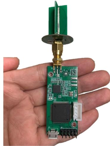
Fig. 9. Self-developed UWB hardware setup which are mounted on parent agents and child agents.
