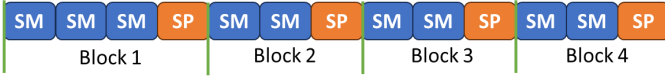
Fig. 7: CenterPoint’s 3D backbone broken into blocks. SM: Submanifold sparse convolution. SP: Sparse convolution.
