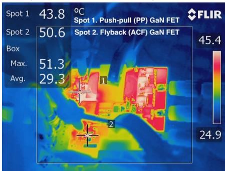
Fig. 15. Thermal Image under Nominal Operation: 28V / 400W
