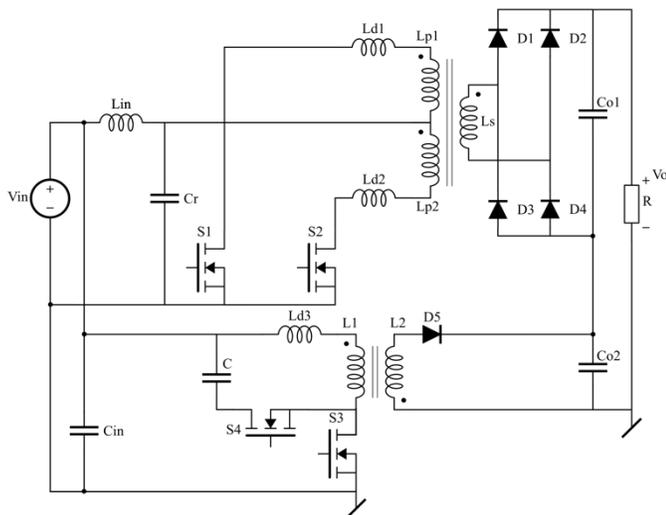
Fig.1. Proposed Circuit Architecture
