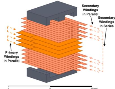
Fig.7. Interleaving Structure
