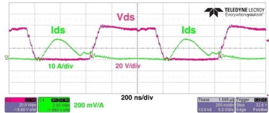
Fig.10. Main Switch Waveforms of Push-pull Converter (PP)
