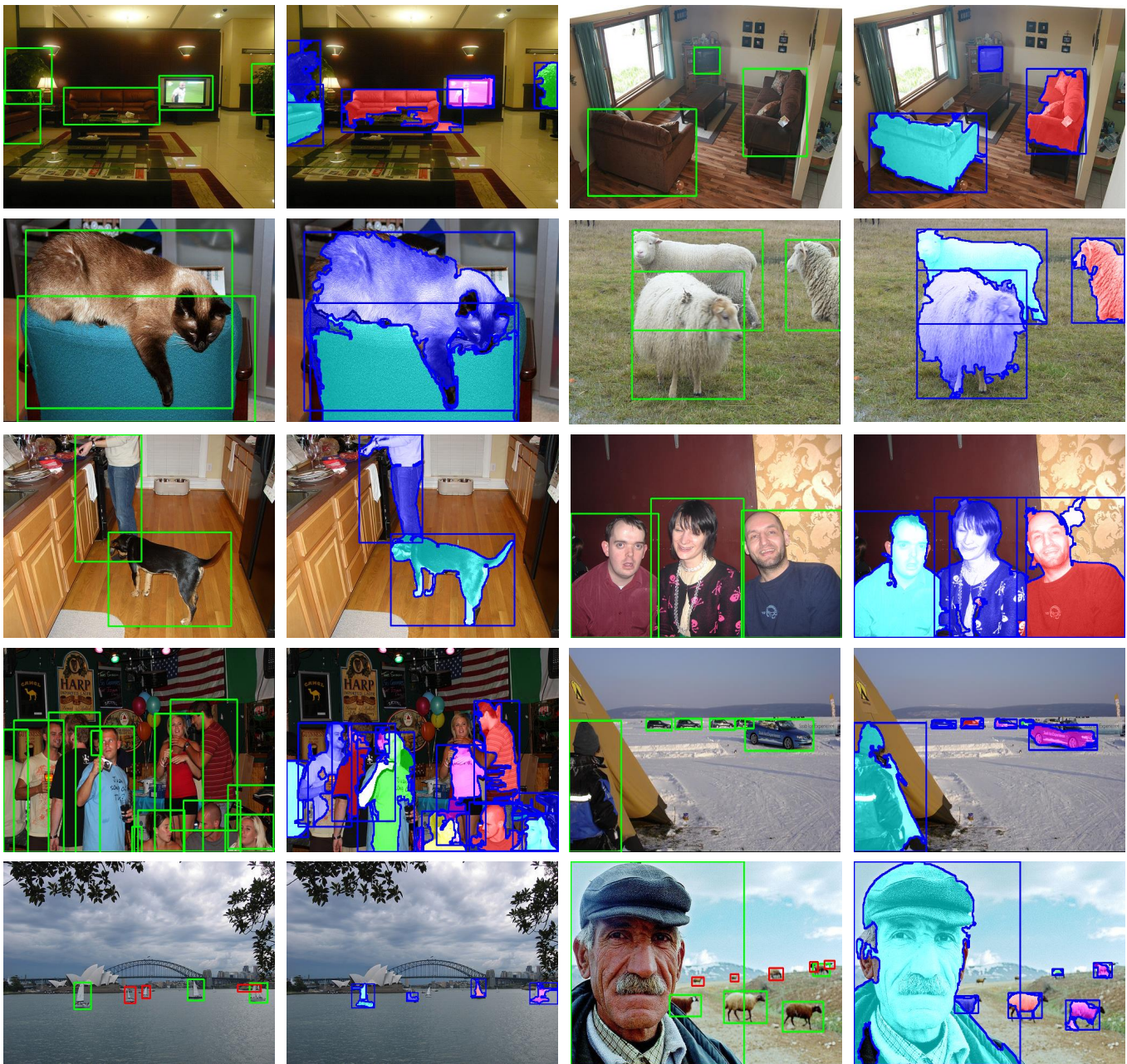
Fig. 8. Qualitative examples of our object proposals. Ground truth boxes are shown in green and red, with green indicating the object is found and red indicating the object is not found. The blue boxes are the object proposals with highest IoU to each ground truth box, and the blue silhouettes are the corresponding object contours. All the samples are taken from PASCAL VOC dataset.
