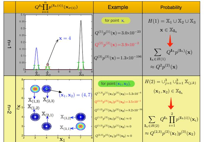
Fig. 1. Example of an MB distribution with three components, and numerical values of the product terms for an  $n = 1$  dimensional hypothesis  $\mathbf{X} = \{4\}$  and an  $n = 2$  dimensional hypothesis  $\mathbf{x} = \{4, 7\}$ . The results show how in each case, regardless of hypothesized dimension, one product term in the sum formed by MB density in (19) becomes much larger than others.
