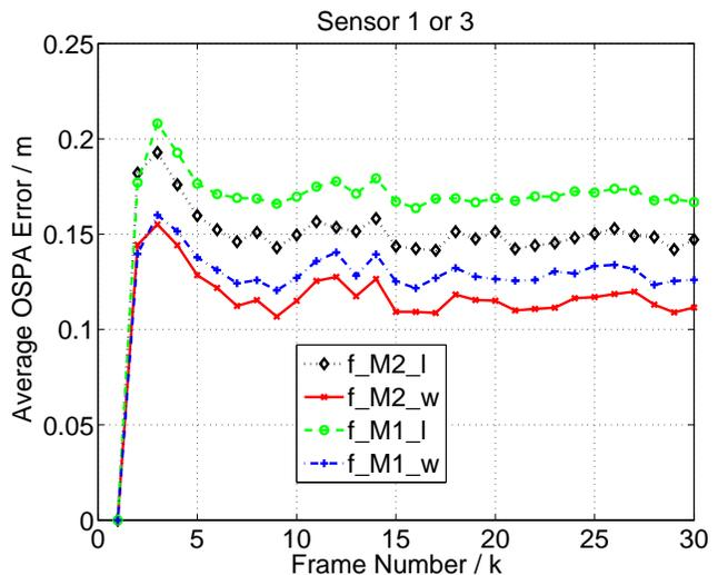
Fig. 10. The average OSPA error of sensor 1 (averaged over 400 MC runs).
