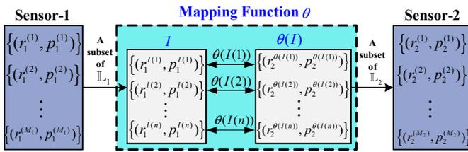
Fig. 2. The sketches of the fusion map defined in Definition 1. For any subset  $I \in \mathcal{F}(\mathbb{L}_1)$ , there is a subset  $\theta(I) \in \mathcal{F}(\mathbb{L}_2)$  whose elements are one-to-one matching with the elements of  $I$ .
