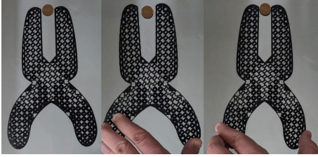
Fig. 16. Fabricated pliers (black TPU). Rest shape on the left; moving the handles apart in the middle; compressing the handles to hold the object on the right.
