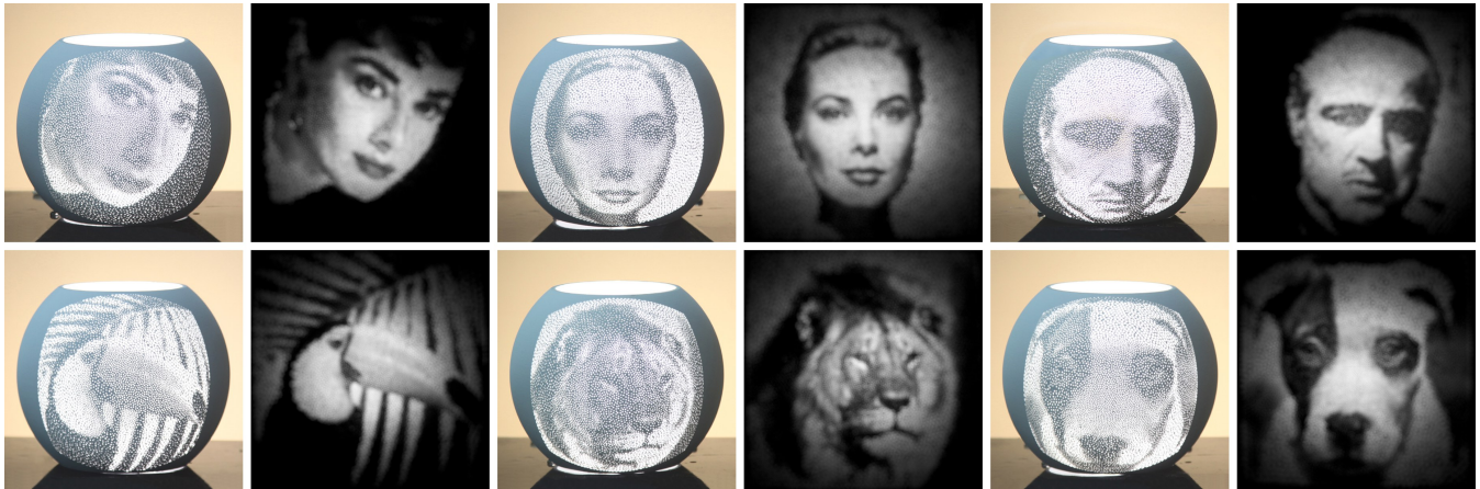
Fig. 11. Additional results on spherical lampshades. Left: our 3D-printed lampshade, with light projecting through the surface. Right: the photo of projected image. The lamps are 22cm in diameter.
