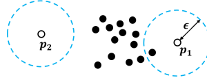
Fig. 1. An example for DBSCAN with MinPts = 4 : the solid points are core points, the point p_1 is a border point, and the point p_2 is an outlier.
