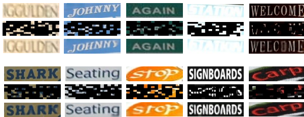
Figure 7: Reconstruction results on images of benchmark datasets. For each column, we show the ground truth (top), the masked image (middle), and the reconstructed image (bottom). The visual masking ratio r_v is set to 0.75.
