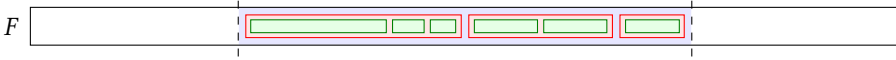
Fig. 3. Clusters are comprised of runs, where all but the first are shifted to the right. A run contains one or more keepsake boxes. The single cluster in the illustration has three runs, and the runs contain three, two, and one keepsake box, respectively.
